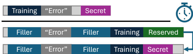
Figure 16: Simplified memory layouts of WebKit’s address space. (Top) No memory pressure is applied. (Middle) Memory pressure is applied with the filler strings, and the target page has not loaded yet. (Bottom) Memory pressure is applied, and the target page has completely loaded.
